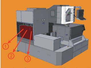
Three filters to extend life cycle and save maintenance cost.
