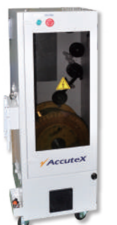
< 45Kg Wire Jumbo Feeder >
