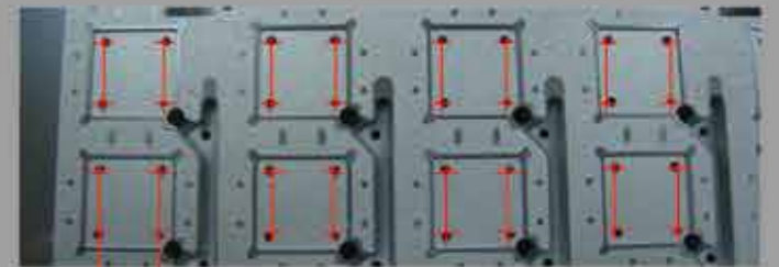
Repeatability 2µm WAFER BUMPING MOLD
